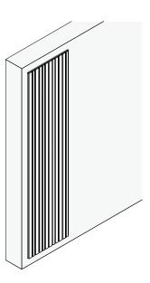
3. With the Timbre panel now located on the wall, apply firm pressure evenly over the entire surface of the Timbre panel. Now, using a countersunk screw suitable for your wall material, place a screw into the felt portion of both upper corners of the panel shown below. Tighten the screw until the head of the screw is flush with the surface of the felt. Repeat this process for both corners at the base of the panel. Your Timbre Panel is now fully installed.
