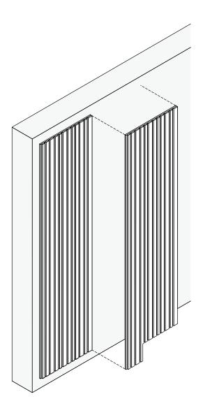
10. With the Timbre panel now located on the wall, apply firm pressure evenly over the entire surface of the Timbre panel. Now, using a countersunk screw suitable for your wall material, place a screw into the felt portion of both upper corners of the panel as show below. Tighten the screw until the head of the screw is flush with the surface of the felt. Repeat this process of both corners at the base of the panel. Your Timbre panel is now fully installed.
