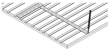
**6.** Now cut the panel along the marked line using a sharp saw blade.
