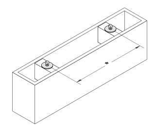
Now, push the Beam onto the hardware mounted on the ceiling, the Beam hardware will 'click' into the ceiling hardware. Your Beam install is complete.
