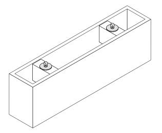
**3.** Mount the female portion of the clips onto the ceiling, using screws to suite your ceiling material. Ensure that the center-to-center location of the female clips match the Beam hardware dimensions.
