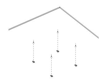
5. Now, push the Bold panel onto the hardware mounted on the ceiling, the hardware will 'click' into the ceiling hardware. Your Bold install is now complete.
