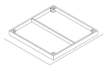
2. Now, locate the EZmark plugs. Insert the plug into the bracket as shown below, ensuring that the plug is pushed firmly all the way to the end of the narrow portion of the slot in the metal bracket.
