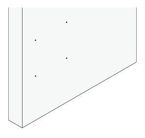
8. Now, remove all the EZmark plugs from the BOLD Wall Panel. The Panel can now be mounted to the wall by aligning the fixings on the wall with the larger hole in the mounting brackets on the back of the Panel. With the Panel against the wall, gently push the Panel down, the Panel will lower by about 19mm (3/4") to seat the brackets securely onto the wall fixings. If the Panel does not lower, adjust the wall fixing screws as necessary.
