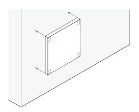
**5.** Using the small markings from the EZmark on the wall as a guide (A), secure your fastener to the wall (B).
