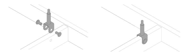
**5.** When all Shoulder-brackets have been installed, your cloud is now complete and ready to be suspended from the ceiling.
