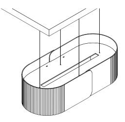
8. Whilst supporting the weight of the LED light unit, secure the light unit suspension points to the ceiling using the Ceiling Hardware
