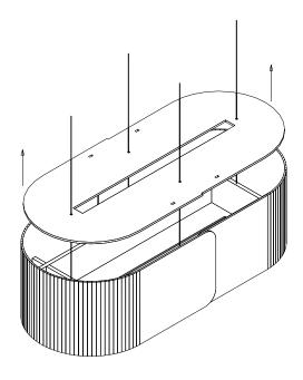
**4.** Place the upper back panel back onto the light shade.
