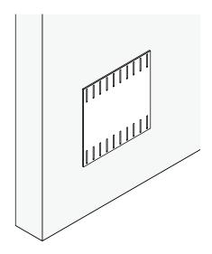
2. On the back-panel tile, starting at the top corner, apply a bead of adhesive that is approximately 1/4" wide. Continue the bead of adhesive across the tile working in a zigzag pattern.
