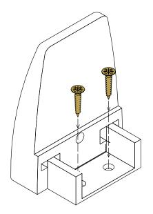
**4.** Place the Desk Divider into the clamps and tighten into place using the bolt provided.
