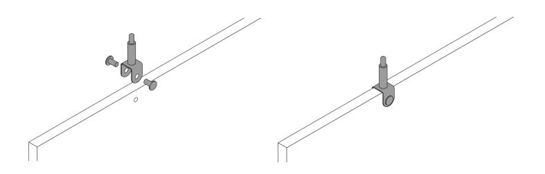
**5.** When all Shoulder-brackets have been installed, your Fin Baffle is now complete and ready to be suspended from the ceiling.
