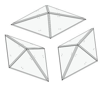
3. Now, apply a small bead of construction adhesive between the pre-marked screw holes on one of the diamond-shaped sections.
