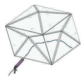
5. Now place the metal bracket over the glue-beads, aligning the holes in the bracket with the pre-marked holes on the cloud sections.
