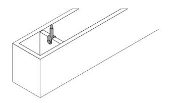
5. Insert the LED light unit into the underside of the Beam. Whilst supporting the weight of the LED light unit, secure the light unit suspension points to the ceiling using the Ceiling Hardware.
