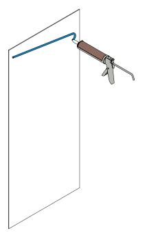
2. On the back of the panel, starting at the top corner, apply a bead of adhesive that is approximately 1/4" wide.
