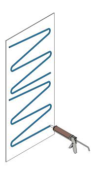
6. With the panel located on the wall, apply firm pressure evenly over the enitre surface of the panel and hold it in place for 30 seconds. The panel is now installed. Repeat steps 1-6 for all remaining panels.
