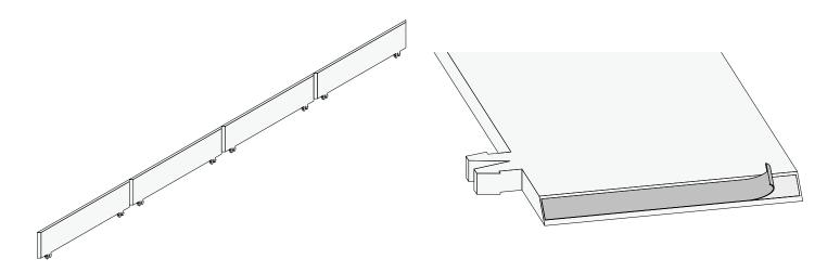
3. Fold the side panel into a square as shown below. Press the joining corners together firmly together to ensure a good bond with the adhesive tape.
